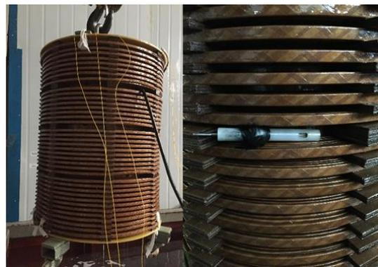
Fig. 9. Test setup and the placement of PD source at the adjacent turns in the high voltage winding as an example
