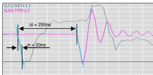
**Figure 6:** Example of a ToF measurement
