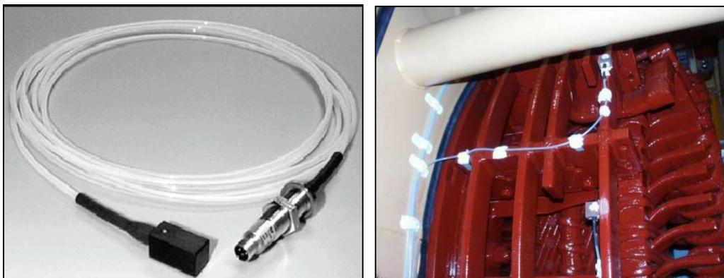
**Figure 9:** Application of fiber optic accelerometers inside a stator end winding basket. The fiber optic accelerometers are non-metallic and do not interfere with the electromagnetic field in the end winding area.
