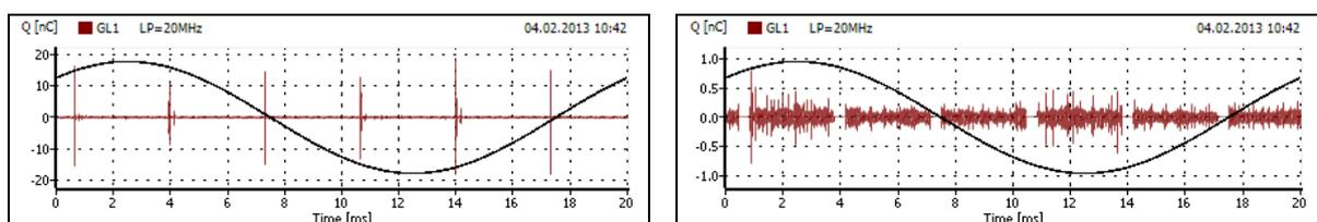
**Figure 7:** Example of an unfiltered (on the left) and filtered signal (on the right)
