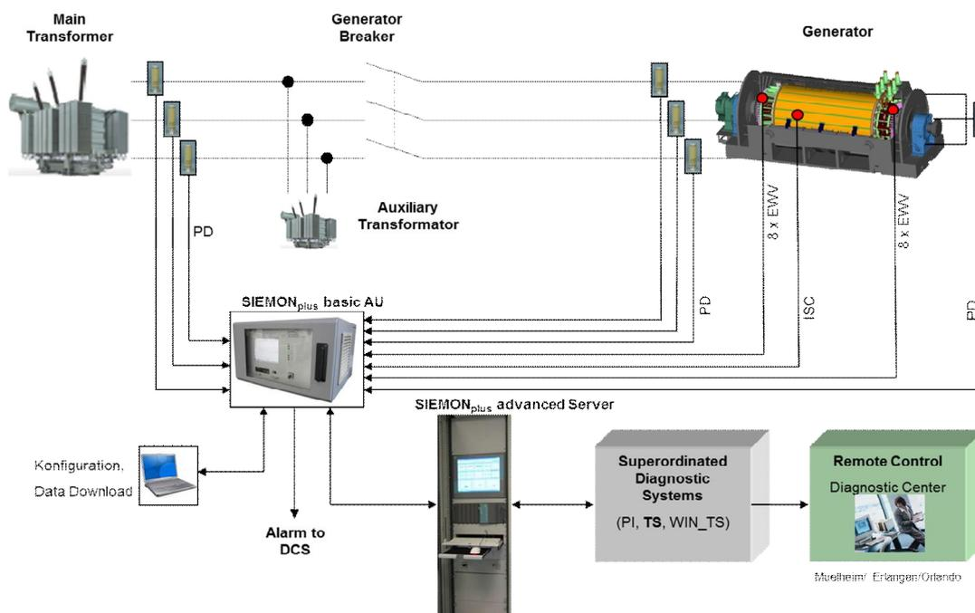
**Figure 1:** Overview of SIEMON<sub>plus</sub> monitoring system
