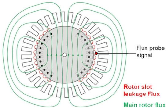
**Figure 13:** Magnetic flux distribution around a two-pole generator
