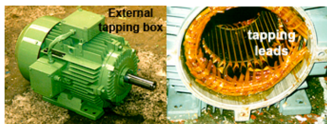
Fig. 1. Left) 11kW low voltage motor used in a test bench for the analysis of inter-turn short-circuits. Right) Stator end-windings showing the leads connected to the stator to cause the fault.
