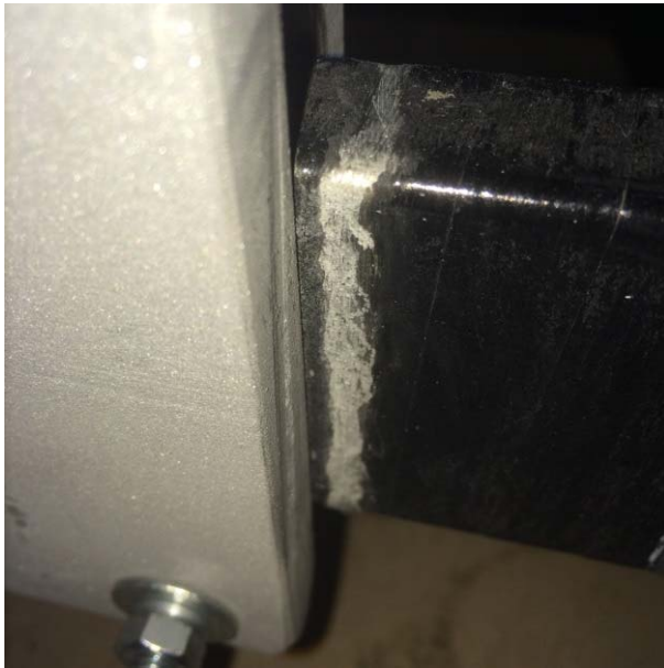
Fig 10. Damage simulation on conducting armour of a resin rich coil rated 11 kV
