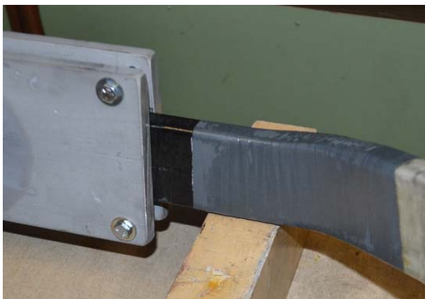
Fig 4: Insulating blocks under stress grading region.
