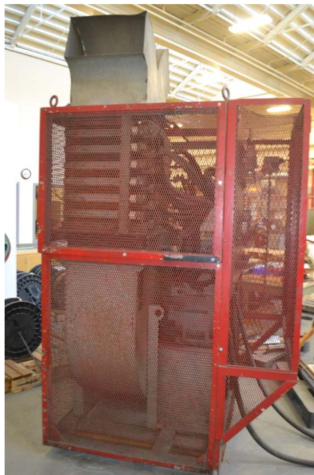
Fig 5: Thermal cycling cell power resistor for controlling current.
